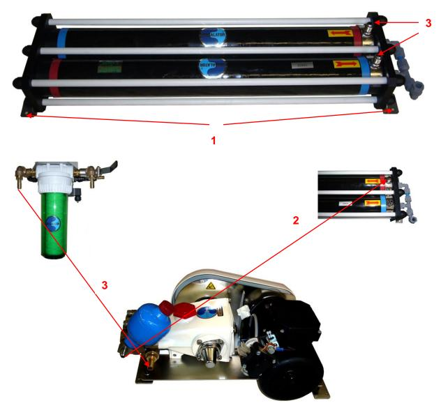
The membranes can be installed horizontally, preferably flat or on a wall support. They are mounted using 8 Parker screws in *stainless steel brackets*<sup>1</sup>. As the hose from the HP pump<sup>2</sup> vibrates, it is preferable to install the hose with an insulating tube. The HP connectors should be installed strictly in accordance with the instructions (Appendix A2). Apply a little loctite or nut seal to the two male and female cones before tightening.
