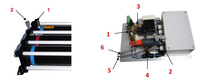
The control panel must be mounted on a vertical surface as close as possible to the motor / pump unit and to the membranes. Leave space behind the panel to facilitate the connections. It is recommended that it is installed at the bottom or on the sides of cupboards, under chart table or main cabin seats, on the front panel of a rear bunk, ...
