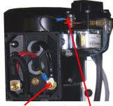
Negative battery cable<sup>4</sup> Positive battery cable<sup>3</sup>. Please connect a fuse holder to this cable. Neutral (blue) phase (brown)
