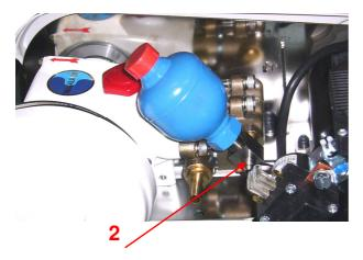
The membranes can be installed horizontally, preferably flat or on a wall support. They are mounted using 8 Parker screws in *stainless steel brackets*<sup>1</sup>. As the hose from the HP pump<sup>2</sup> vibrates, it is preferable to install the hose with an insulating tube. The HP connectors should be installed strictly in accordance with the instructions (Appendix A2). Apply a little loctite or nut seal to the two male and female cones before tightening.
