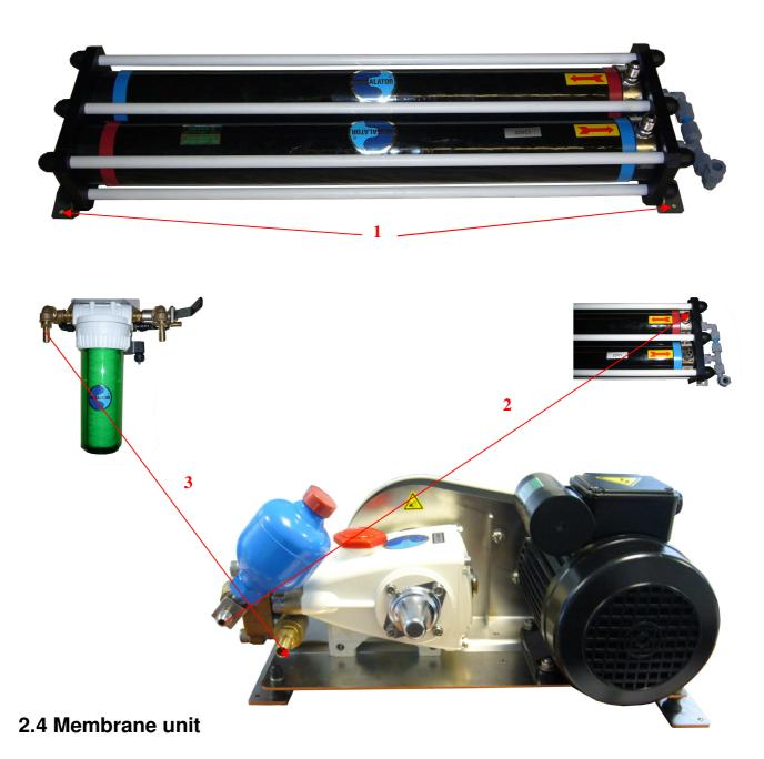
The membranes can be installed horizontally, preferably flat or on a wall support. They are mounted using 8 Parker screws in *stainless steel brackets*<sup>1</sup>. As the hose from the HP pump<sup>2</sup> vibrates, it is preferable to install the hose with an insulating tube. The HP connectors should be installed strictly in accordance with the instructions (Appendix A2). Apply a little loctite or nut seal to the two male and female cones before tightening.
