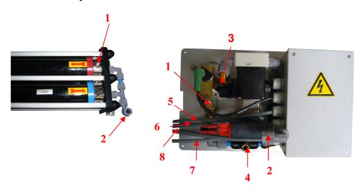
The control panel must be mounted on a vertical surface as close as possible to the motor / pump unit and to the membranes. Leave space behind the panel to facilitate the connections. It is recommended that it is installed at the bottom or on the sides of cupboards, under chart table or main cabin seats, on the front panel of a rear bunk, ...
