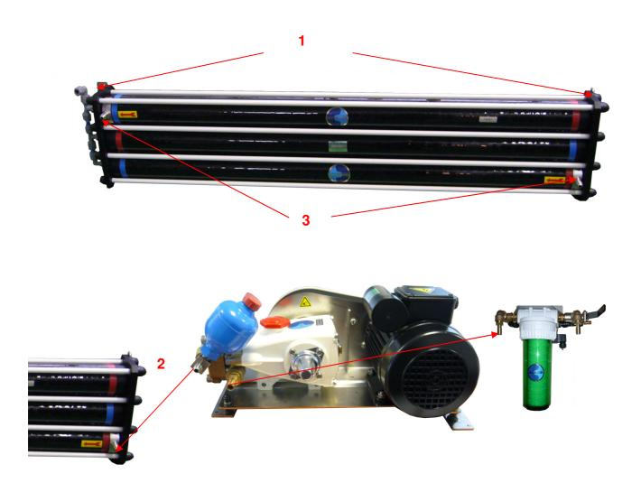
The membranes can be installed horizontally, preferably flat or on a wall support. They are mounted using 8 Parker screws in *stainless steel brackets*<sup>1</sup>. As the hose from the HP pump<sup>2</sup> vibrates, it is preferable to install the hose with an insulating tube. The HP connectors should be installed strictly in accordance with the instructions (Appendix A2). Apply a little loctite or nut seal to the two male and female cones before tightening.
