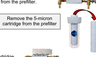
Replace it with the sterilizing cartridge
