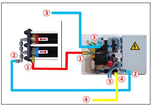
**1** Hose for connecting the high-pressure membrane outlet to the high-pressure control valve on the back of the front panel. (Black high-pressure hose supplied)
