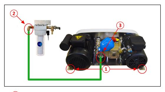
(1): Stainless steel legs for fixing the motor/pump block
