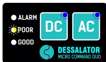
The RED, YELLOW and GREEN LEDs will show the same indication as on the control panel of the watermaker.
