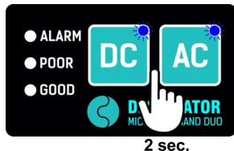
To start the watermaker from STANDBY and run it on DC power, press and hold **DC** for about 2 seconds.
