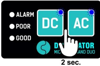
To start the watermaker from STANDBY and run it on DC power, press and hold **DC** for about 2 seconds.
