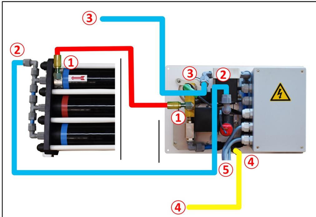
① Hose for connecting the high-pressure membrane outlet to the high-pressure control valve on the back of the front panel. (Black high-pressure hose supplied)
