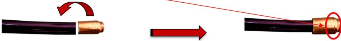
2. Place the brass plug in the stainless steel nut and tighten it firmly:
