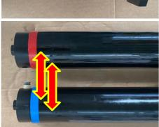
Separate the membranes to remove the inter-connector(s), be careful not to damage the O-rings.
