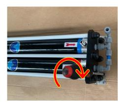
Return the membrane block to its original place and using a screwdriver, screw the 8 fixing screws of the membrane block back
