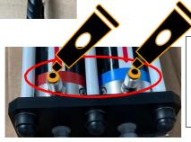
Use threadlocker such as Loctite 542 liquid or 577 paste only on the lip of the 2 males connectors (membrane block side) before assembling the high pressure pipe connectors on those of the membrane block.
