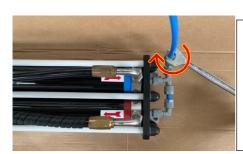
Put the blue hose ø10mm back into the Serto fitting and with a flat wrench n°17, screw the fitting back in.
