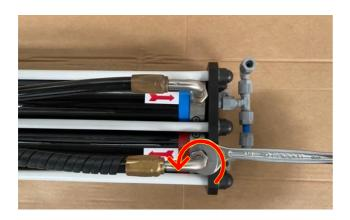
With a flat wrench n°19, unscrew the fittings of the 2 high-pressure pipes.
