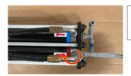
With a flat wrench n°19, screw the connections of the 2 high-pressure pipes back to those of the membrane block.
