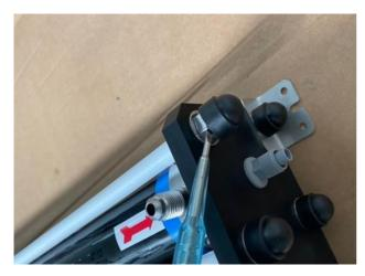
With a small flat screwdriver, remove the nut aps on each side of the 2 flanges.
