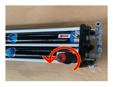
Using a screwdriver, unscrew the 8 fixing screws of the membrane block
