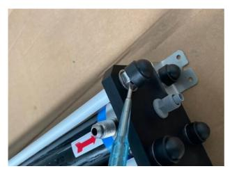
With a small flat screwdriver, remove the nut caps on each side of the 2 flanges.
