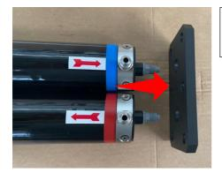
Remove the flanges on each side of the membranes.
