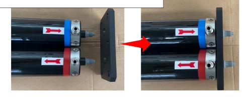
Replace the tie rods that hold the 2 flanges.
