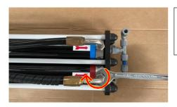
With a flat wrench n°19, screw the connections of the 2 high-pressure pipes back to those of the membrane block.
