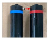
Replace the flanges on each side of the membranes.
