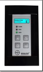
**<u>Restarting the watermaker</u>**: Use the button on the Mini Remote Control until you hear 2 beeps. At that moment, you can:
