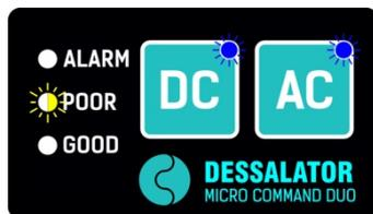
The RED, YELLOW and GREEN LEDs will show the same indication as on the control panel of the watermaker. The blinking speed of the YELLOW LED provides feedback of the water pressure in the system : faster blinking means higher pressure. The BLUE LED that is lit shows if the machine is running on DC or AC power. Once the production water is of good quality, the GREEN LED will light up.
