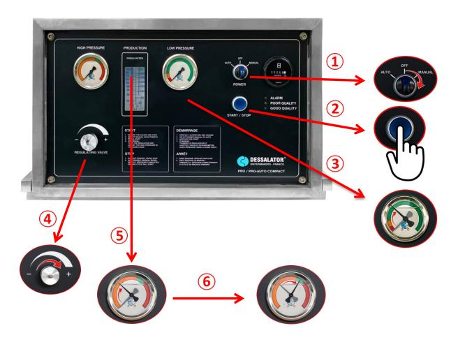
$\rightarrow$ Note : Too high a pressure setting stops the watermaker and turns on the red light. In this case, decrease the pressure with the pressure regulation knob ④ and repeat the startup procedure.
