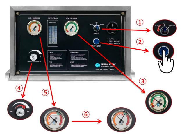
→Note : The fresh water yield depends on the temperature and salinity of the sea water and the cleanliness of the 5 & 25 micron filters (in the pre-filter).
