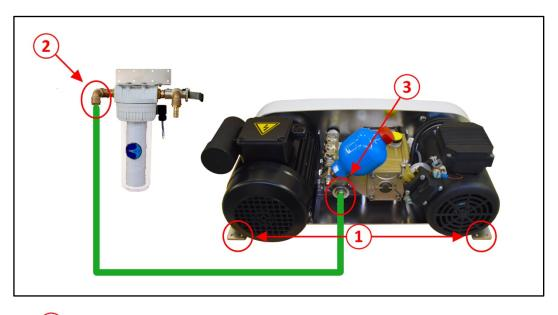
(1): Stainless steel legs for fixing the motor/pump block
