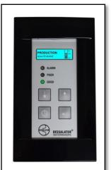
Restarting the watermaker: Use the button on the Mini Remote Control until you hear 2 beeps. At that moment, you can:
