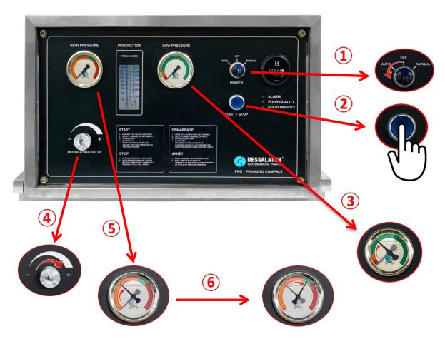
→ Note: The fresh water yield depends on the temperature and salinity of the sea water and the cleanliness of the 5 & 25 micron filters (in the pre-filter).
