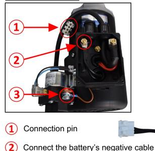
3 Connect the battery's positive cable (do not forget to install the fuse holder)
